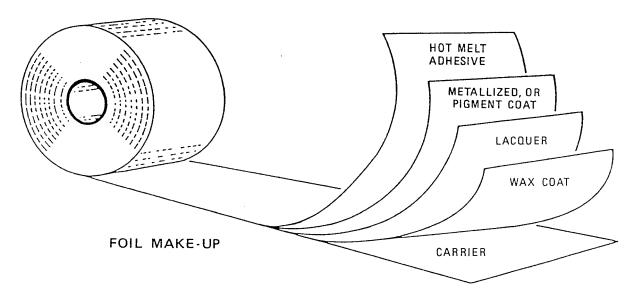
Hot stamping foil, roll-leaf, or tape, as it is often referred to, is comprised of a carrier film and various heat reactive coatings. An image or design is transferred from the foil by the application of pressure and heat to the carrier material for a brief duration (referred to as dwell) normally less than a second; temperature is determined by the foil composition and the material it is being applied to.
